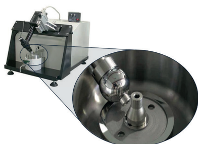
Figure 1 Mini Traction Machine with magnified steel ball against steel disc configuration
