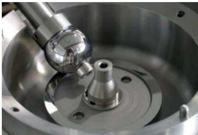
Figure 4 Mini Traction Machine set up in a ball-on-disc configuration
