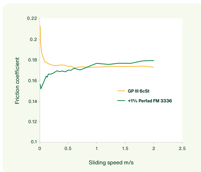
Graph 3: Change in the friction of a mineral oil by the addition of Perfad™ FM 3336 friction modifier on a steel-clutch paper contact.
