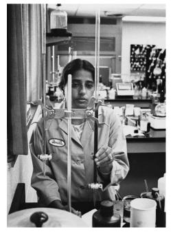
Employee Shindi Mahal, lab technician, tests the sulphur dioxide content of corn syrup at a corn milling plant in Dayton, Ohio, 1973.
