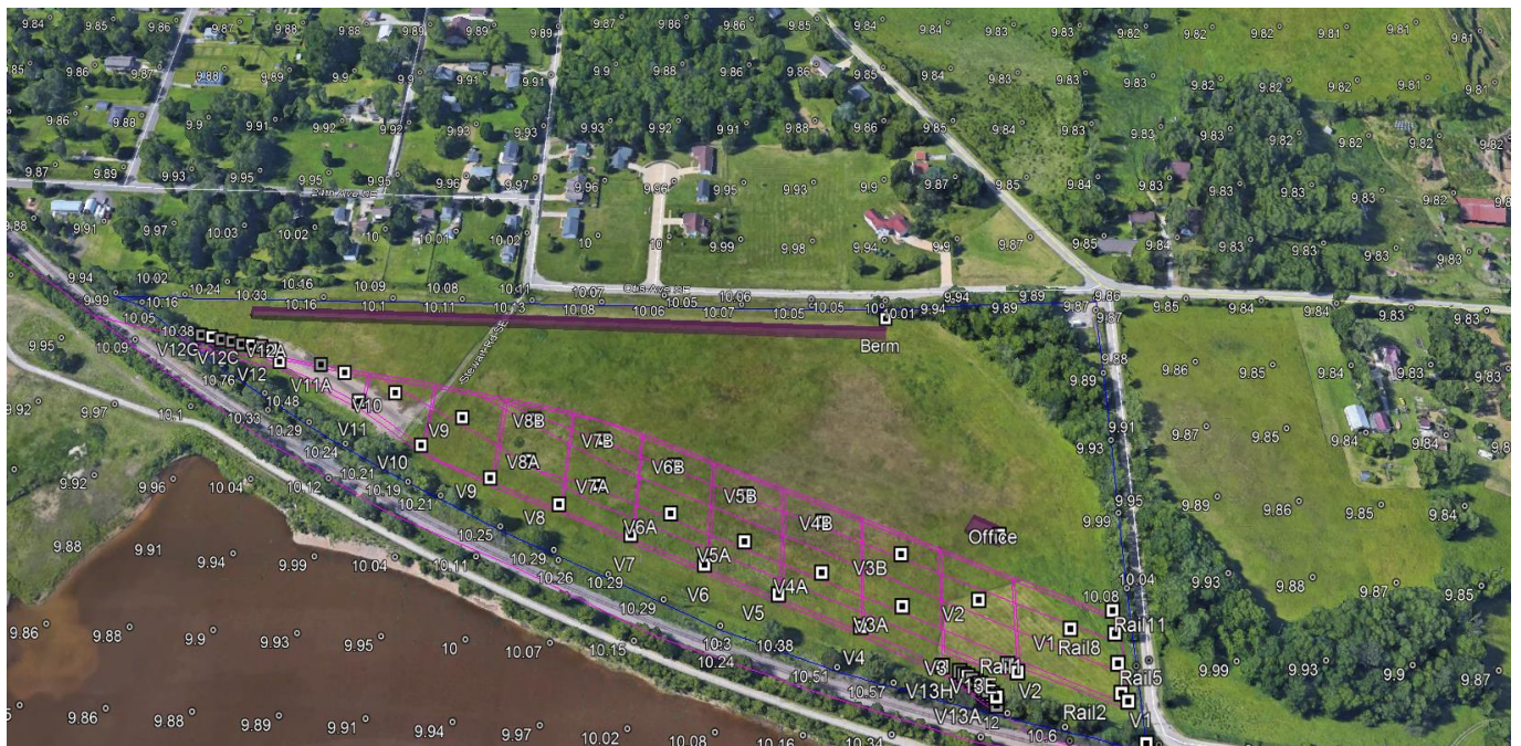
Figure 6. PM2.5 Annual Result Distribution. High value of 12 ug/m3 is along south property line. Results along north property line 10 ug/m3 or below.
