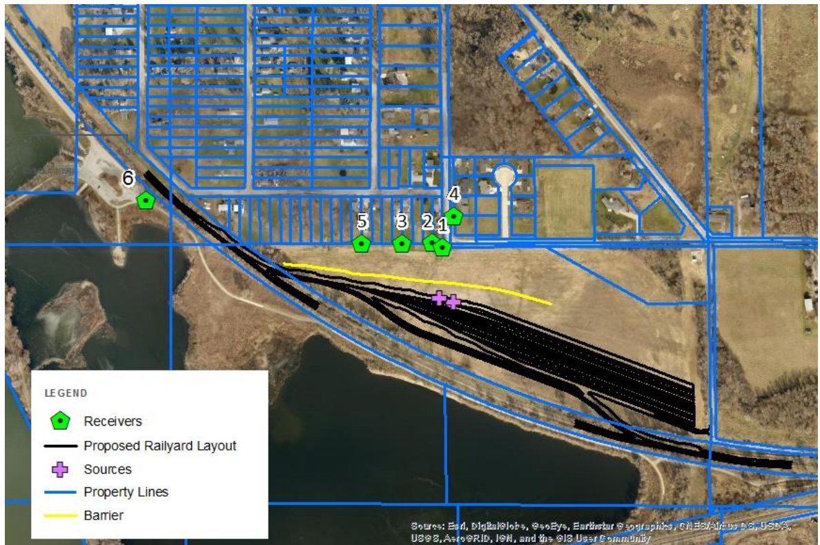
Figure 3 Location of Modeled Noise Barrier near Northern Rail Line
