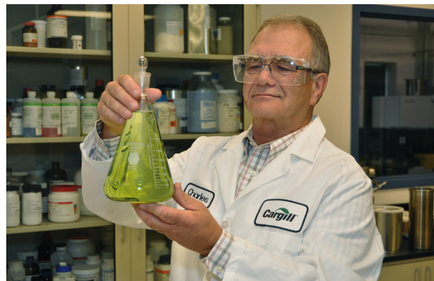
The dielectric fluid is a natural ester and has been classified as carbon-neutral by the BEES 4.0 life-cycle analysis.
