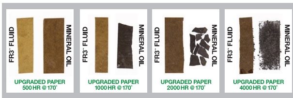
Figure 1 - Thermally upgraded paper accelerated aging in FR3 fluid and mineral oil side-by-side comparison. Cooper Power Systems ML-152-2000.
