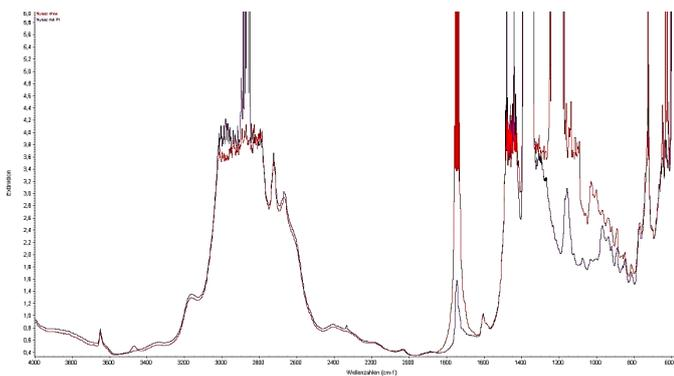
Figure 7: FTIR Spectrum - Nynas Transformer Oil Nytro 4000X – Modification after treatment (ageing)
