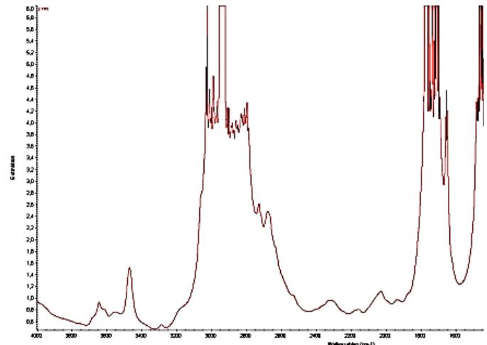
Figure 8: FTIR Spectrum - Natural Ester – Envirotemp™ FR3™ Before Ageing
