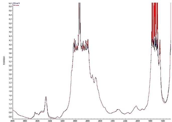
Figure 9: FTIR Spectrum - Natural Ester Envirotemp™ FR3™ - Modification after treatment (ageing)
