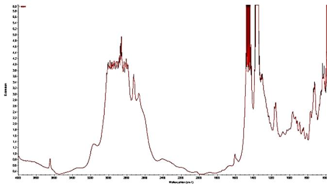
Figure 6: FTIR Spectrum - Nynas Transformer Oil – Nytro 4000X Before Ageing
