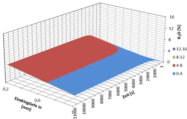
Figure 4: FR3<sup>TM</sup>, 1,5% – moisture in pressboard – envelope
