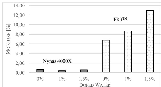
Figure 2: Water content of the insulating liquids after treatment
