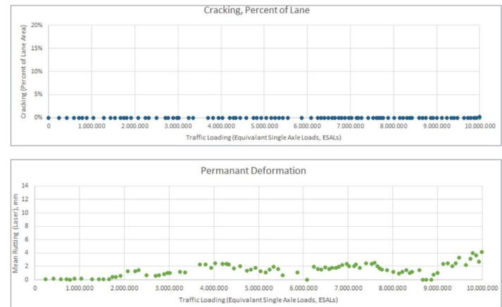
Figure 2 Field performance from monitored NCAT test section after 10 million ESALs of loading
