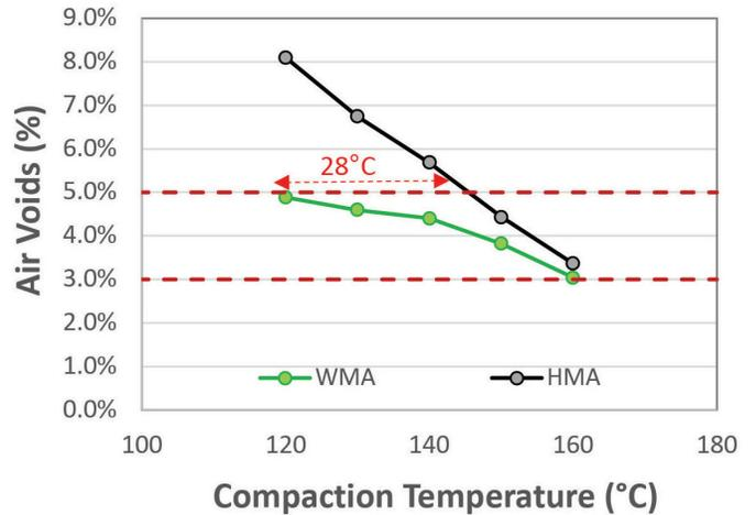
Figure 1 Impact of reduced compaction temperatures on achieved mixture air voids
